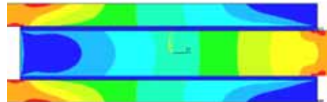
Fig. 11 Equivalent stress distribution.
