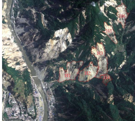
Fig. 8 Identified landslides as loose deposits of the Hongchun Gully debris flow. H is the abbreviations of landslides.
