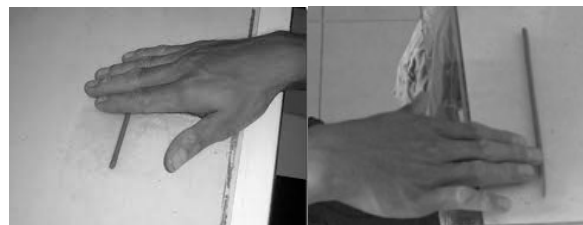
Fig. 1 Rolling thread method.
