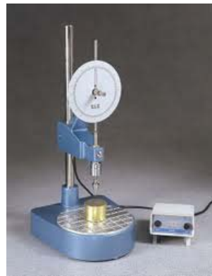
Fig. 2 The fall cone test are used during the experiment.
